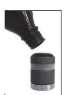
The electrodes must not be touched with fingers Do not remove the coating on the electrode
