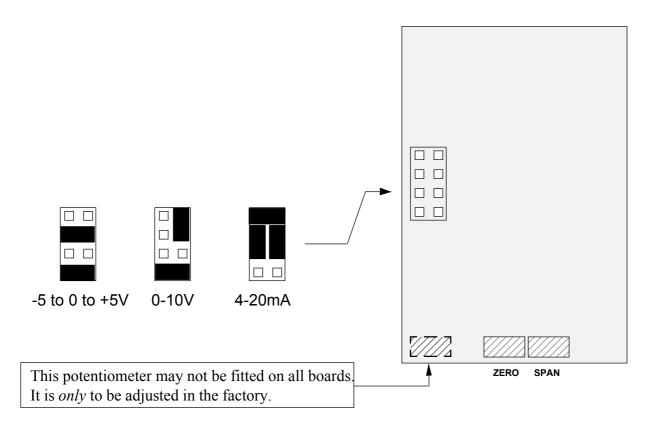
Re assemble the meter, apply power and follow the Analogue Output Settings procedure on the next page. Measure the analogue output and trim, if needed, using the ZERO and SPAN potentiometers, for best accuracy.
