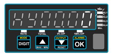
The hysteresis value is directly related to your measurements, so, for example, if you have a high alarm, set to 500, and set the hysteresis value to 7, the alarm will occur when the meter reading rises above 500, and will reset when the meter reading falls to 493.
