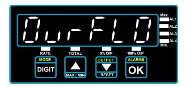
"Overflow" = The counter has reached or exceeded its capacity of 999999. If this occurs earlier than desired, consider dividing the count by 100, or 1000 and use either 2 or 3 decimal places, and label the reading 'X 100' or 'X 1000'
