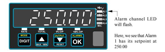
To change alarm settings, select the alarm you wish to change as shown above until its LED is flashing, then press the ALARM key for more than 3 seconds. You will see one digit is brighter than the others. You can change its value using the UP/DOWN buttons, and then select other digits with the DIGIT SELECT pushbutton. When the value has been set, press OK.
