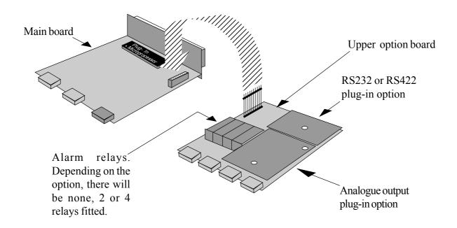
The analogue output and RS232 or RS422 plug-in option boards are fixed to the upper option board with white plastic pillars. You must apply a firm force when fitting or removing these options.
