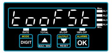
"Too Fast" = The input signal frequency is higher than the meter can accept. Reduce input frequency or use a signal source (encoder etc.) with lower output rate.
