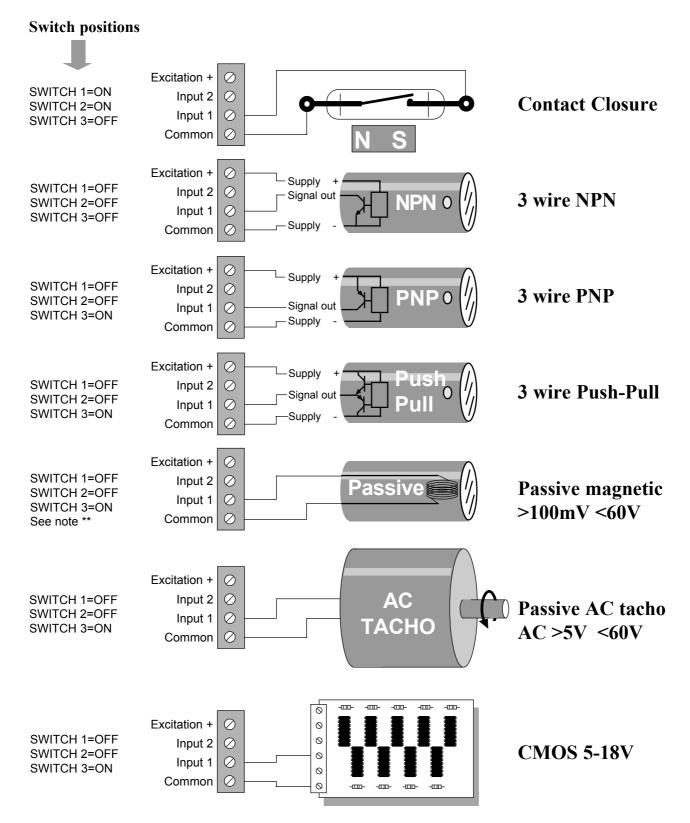
\*\* To activate the internal amplifiers, required for low level signals, it is necessary to fit a pair of jumpers on the gold pins marked S5( for I/P2) and S7 ( for I/P 1). These pins are located inside the meter, 30mm in front of the Input connector. Please see the page 'How to Install Option boards' for advice on opening the case.
