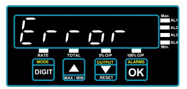
"Error" =Microprocessor error. There may be a fault in the meter, or the meter has been unable to perform a computation. The scale factor may be set to a value beyond the capability of the meter.
