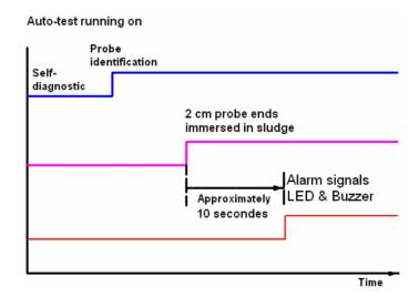
The test could be completed with the probe outside the separator and totally immersed in water. After the self diagnostic sequence, the control unit recognized the sludge probe and will:
